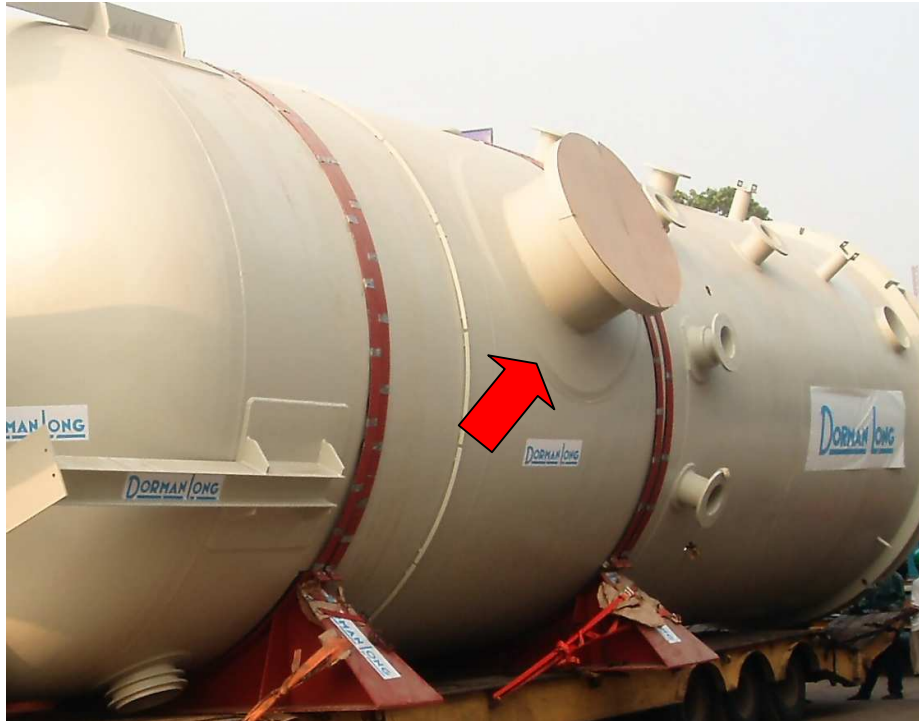
Figure 1 – Typical example of a part with strengthening
